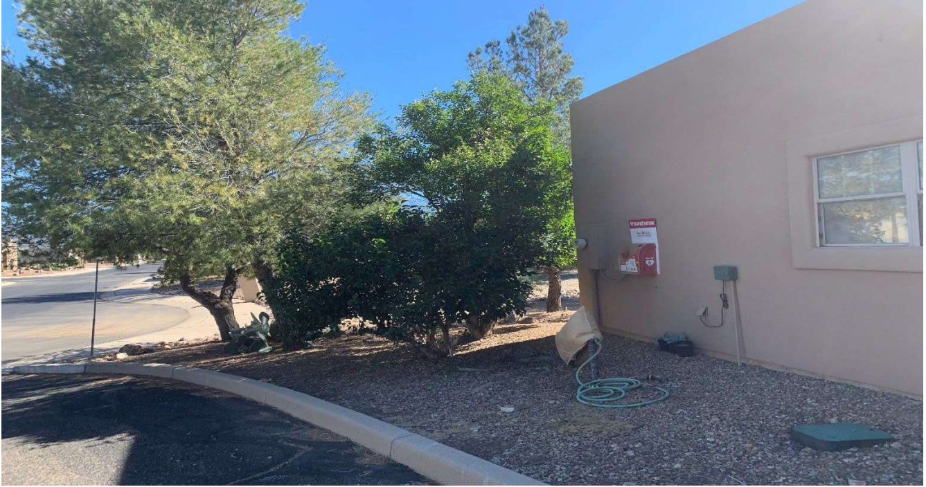
Vegetation in the Intermediate zone. Keep separation of Trees/ Bushes around 5' along with grass trimmed.
